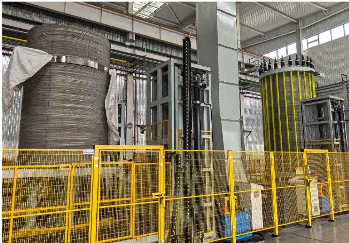
Alkaline electrolyzer production line
